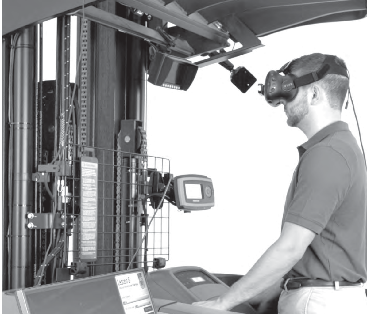
This simulator is a virtual reality headset that can plug into the newer Raymond forklift. When plugged into the forklift the headset automatically generates a simulation for the driver to train on. (Submitted photo)
